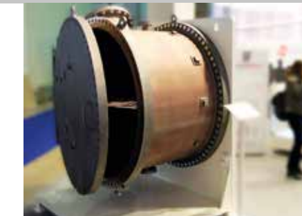
Water box CuNi 90/10
