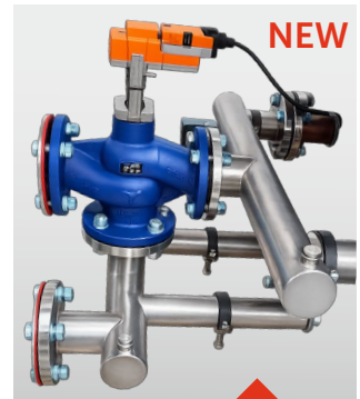
3 Way Valve A three-port valve that controls and diverts the flow of water between the free cooler and the chiller. Supplied with connection manifolds for easy chiller integration, it automatically switches to free cooling when conditions allow, reducing energy consumption.
