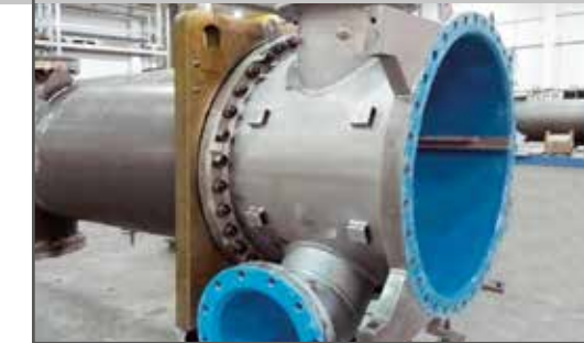
Water box epoxy coating
